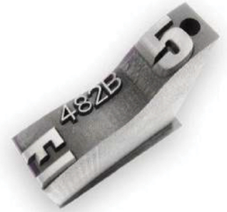
3D yüzeye 2D derin kazıma 2D deep scraping on 3D surface
